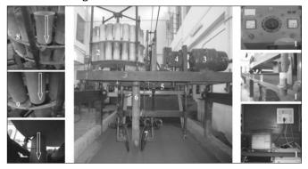
Fig. 11. Multistage rotating cup metering mechanism (44).
