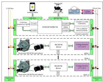
Fig. 13. GPS based Seed metering control system (61).
