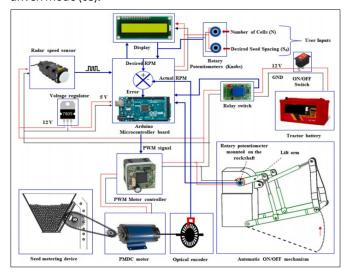
Fig. 15. RADAR based mechatronic seed metering control system (63).
