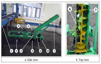
Fig. 12. The Auger-type metering device (45).
