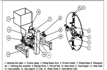
Fig. 10. Automatic ginger metering mechanism (41).
