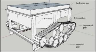
Fig. 14. Autonomous planting robot (62).
