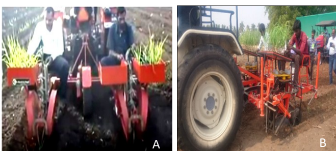
Fig. 14. Settling transplanting. (A) Chain sugarcane transplanter, (B) Cup type sugarcane transplanter.
